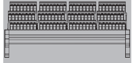
Field terminals view for ADV161 (Channels 33 to 64)
