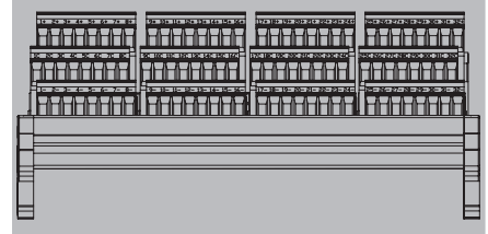
Field terminals view for 1384350000 (ADV151)
