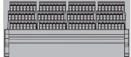
Field terminals view for ADV161 (Channels 33 to 64)
