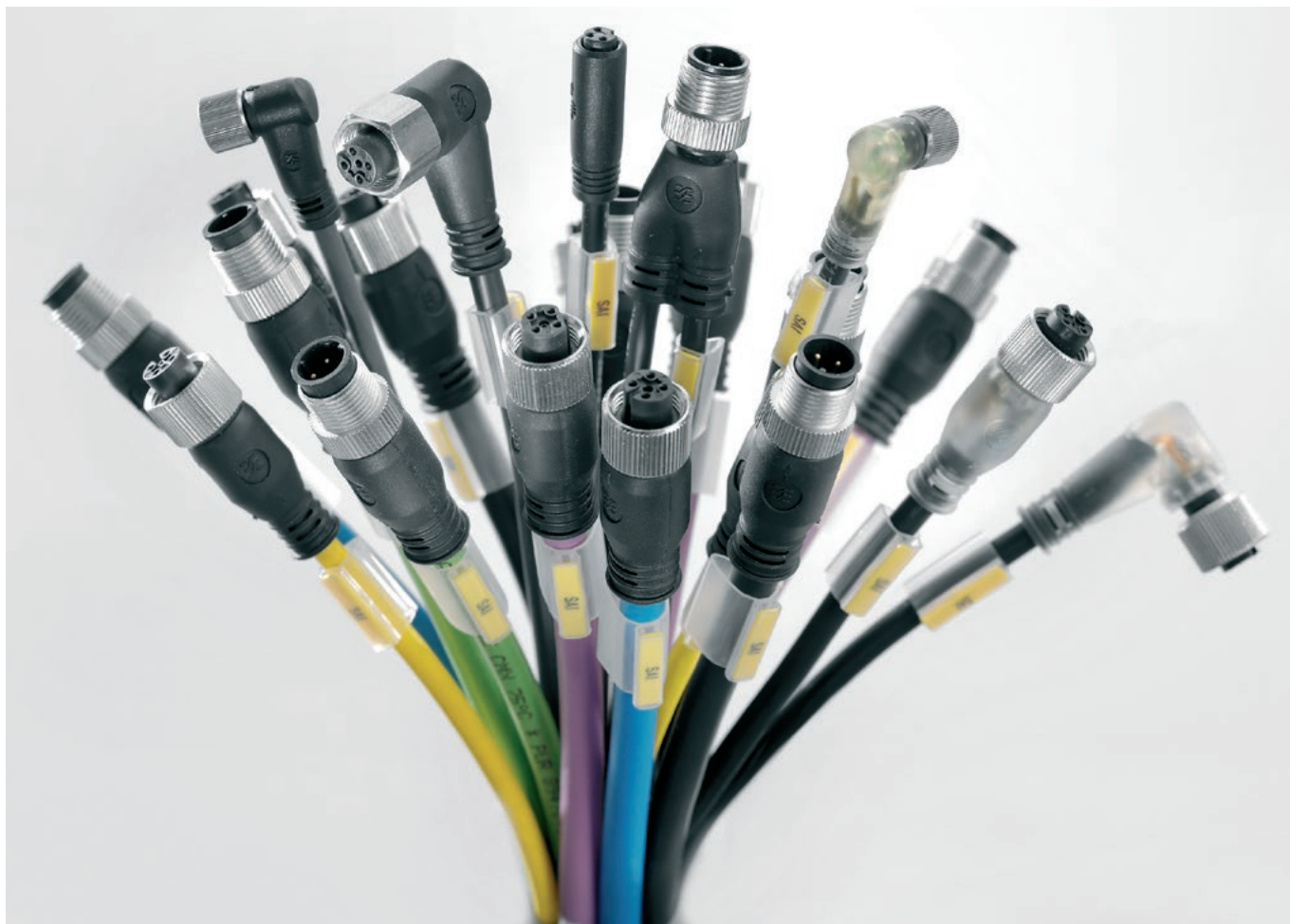
Bus cables: shown here in the standard colours: blue (Profibus-PA Ex i), black (CANopen/DeviceNet or Profibus-PA), magenta (Profibus-DP) and green (Industrial Ethernet) together with the sensor cables
