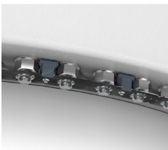
Detection plates for measuring and holding back broken bolts on the rotor blade bearing
